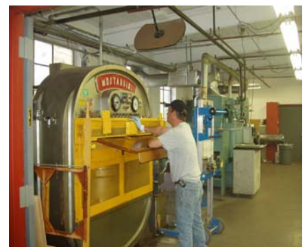
A ProtoLab project leader fits a coated sheet into the embossing machine.
